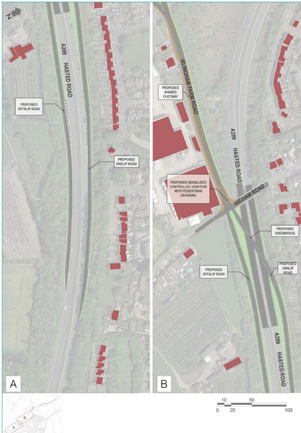
Figure 3: Phase 1 - Modifications to A289 including providing new slip roads to Higham Road junction, new overbridge, improvements to Islingham Farm Road and Woodfield Way
